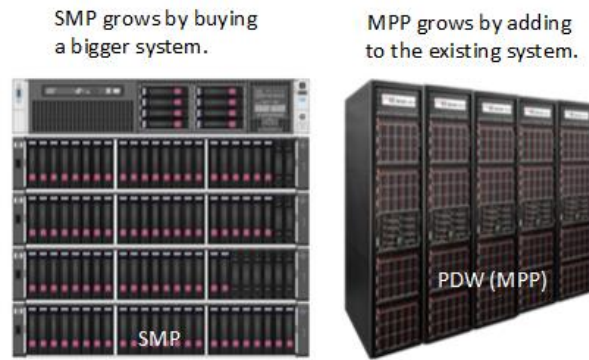
Figure 3: Scalability of today's SMP systems compared to PDW's MPP design
