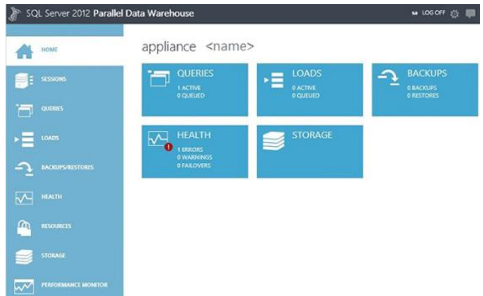
Figure 1.2: PDW has a web-based Admin Console for monitoring the appliance.
